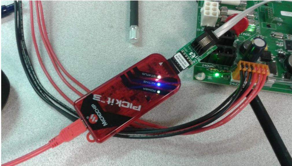
Programming of the CPU board is complete when the "Status" LED is illuminated green and the blue "Active" LED is blinking.
