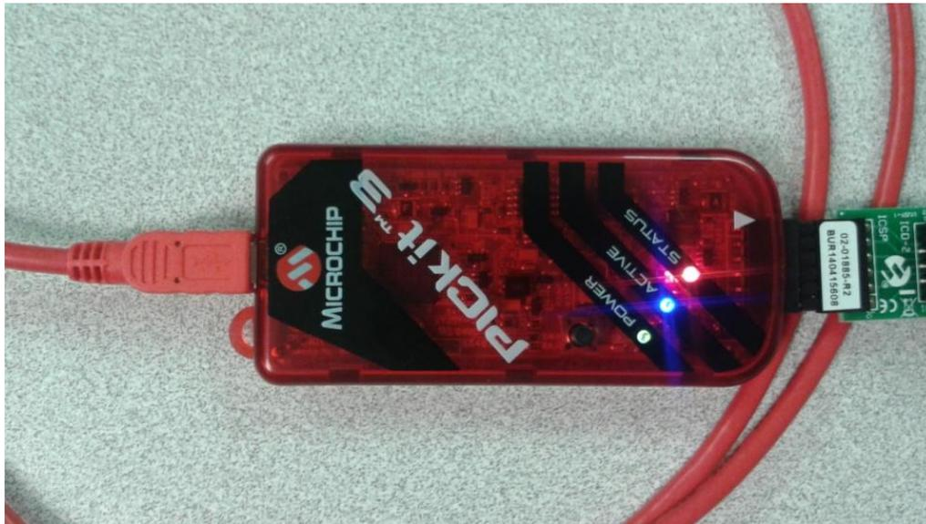
After a few seconds to as much as twenty seconds, the "Status" LED will be off and the blue "Active" led will be blinking. The PicKit3 is now ready to program the device.
